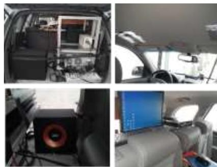
Fig. 9 Equipment for the active noise control of interior noise in the test vehicle.
