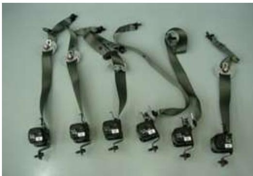
Fig. 13 Seat belt component for 6 seat belt samples used for the improvement test of the emotional feeling about the fastening force of a seat belt
