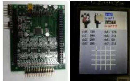
Fig. 3 Signal processing and filter controller
