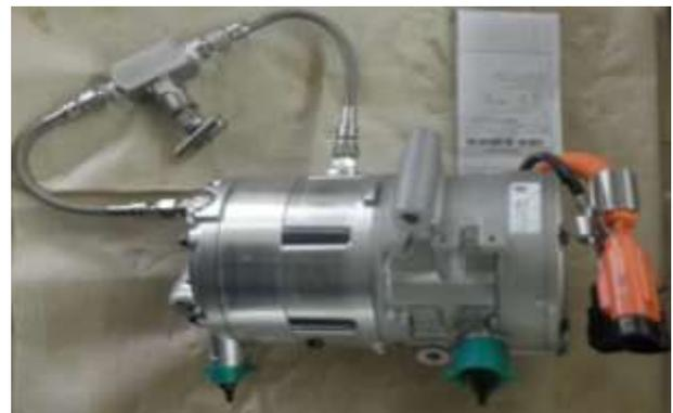
Fig. 3 Modified e-Comp. to determine target back pressure
